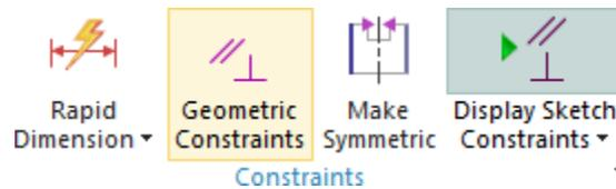
The **Geometric Constraints** dialog box behaves differently from most other dialog boxes in NX – there is no **OK** button and no **Apply** button. You simply select the constraint you wish to apply, then click on the object(s) you wish to constrain. Once you have specified at least one **Object to Constrain**, and one **Object to Constrain to**, the constraint is applied and the menu resets.
