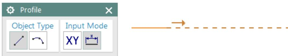
The thickened bar in the middle of the line segment is the **Horizontal** constraint.
