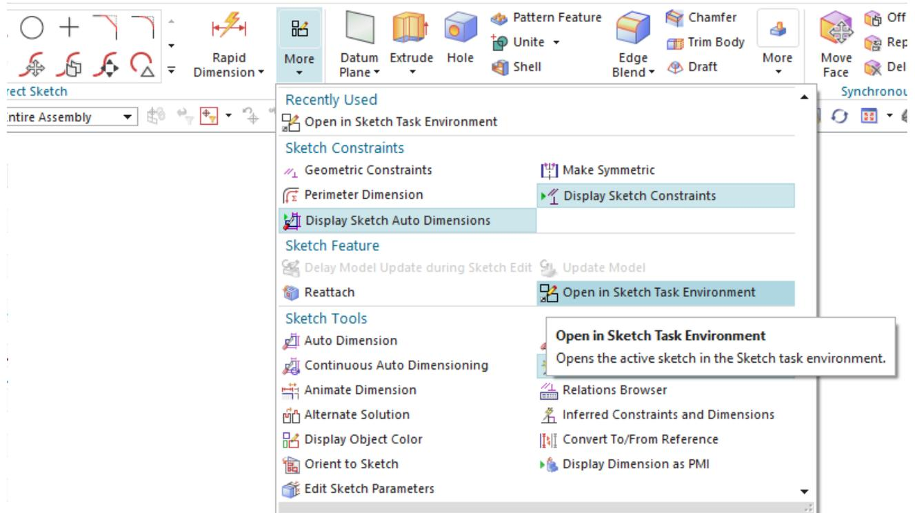
When sketching in the **Task Environment**, the ribbon changes completely – most tabs disappear, and **File** becomes **Task**. Additionally, the entire **Home** tab is populated with sketch-specific tools. Their names are displayed, too!
