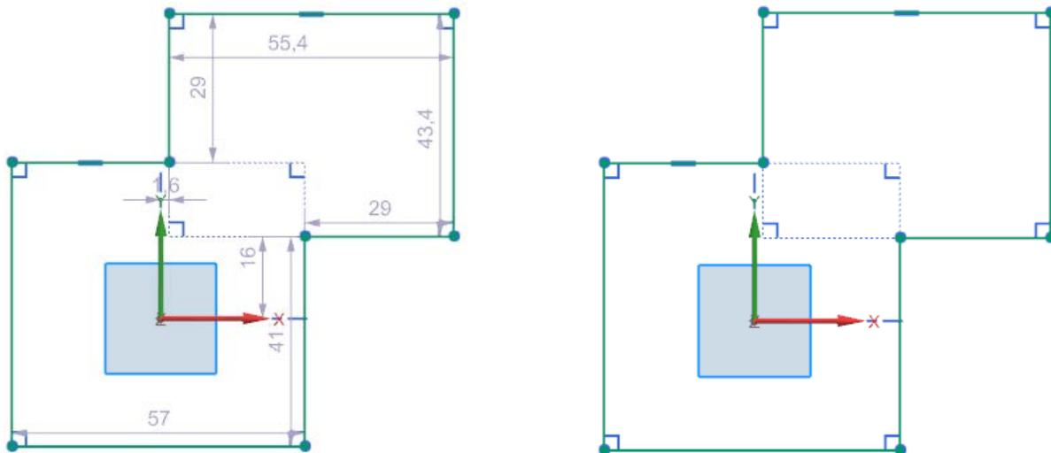
The dimensions placed when **Continuous Auto Dimensioning** is enabled are “weak” or *driven* dimensions, rather than *driving* dimensions – they can be overwritten by other constraints and dimensions and will not conflict with those other constraints. However, they are sometimes more difficult to edit, and tend to give sketches a cluttered appearance.
