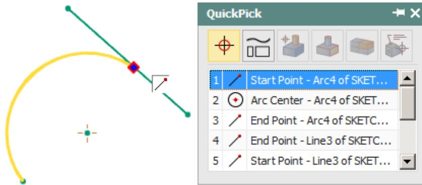
Control points are useful for a variety of tasks, such as building new geometry or making measurements of existing geometry. NX 11 is sensitive to how you pick curve entities and may provide different results based on whether you select the curve itself or its control points.
