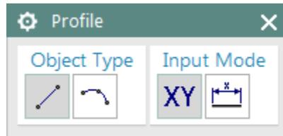
The **Profile** tool combines the essential functionality of the **Line** tool with that of the **Arc** tool. You can choose whether you would like a line segment or an arc by clicking on the corresponding icon in the **Object Type** section of the Profile dialog box, or you can switch back and forth between arcs and lines more fluidly as follows:
