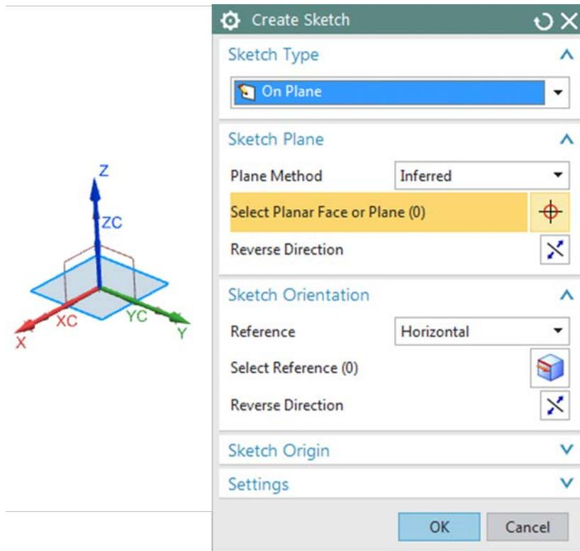
2. Orient your sketch the way you want it. When the **Create Sketch** dialog box is open and your cursor hovers over a face, the red-blue-green coordinate system that appears gives a preview of the sketch coordinate system's location and orientation. For example, clicking on the upper right corner of the face shown below will orient the sketch coordinate system as indicated.
